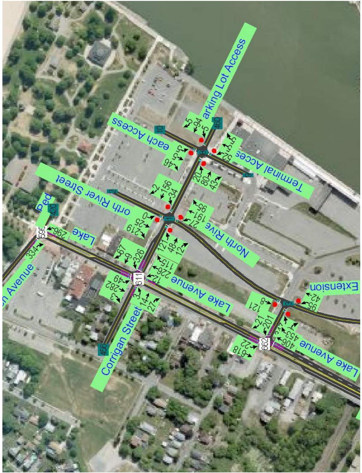
2020 Build Saturday 3:30 – 4:30 PM Peak Hour Intersection Turning Movement Volumes With North River Street Connection between Corrigan Street and Portside Drive
