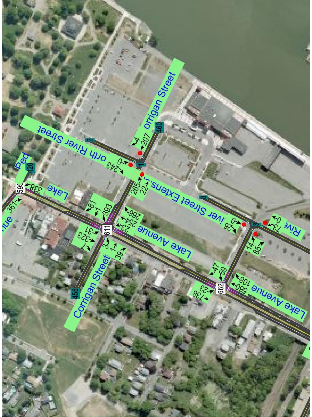
2020 Build Friday 8:30 – 9:30 PM Peak Hour Intersection Turning Movement Volumes No North River Street Connection between Corrigan Street and Portside Drive
