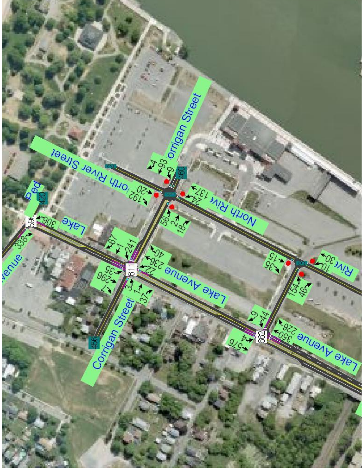
2010 Existing Friday 8:30 – 9:30 PM Peak Hour Intersection Turning Movement Volumes With North River Street Connection between Corrigan Street and Portside Drive
