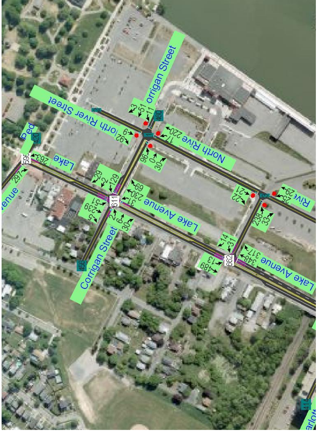
2010 Existing Friday 6:30 – 7:30 PM Peak Hour Intersection Turning Movement Volumes With North River Street Connection between Corrigan Street and Portside Drive
